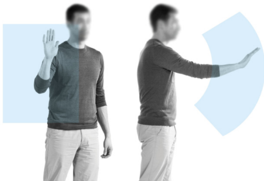
Figure 1: The physical interaction zone is the volume inside which hand movements lead to meaningful interactions (Fig. modified from [Mic14])
