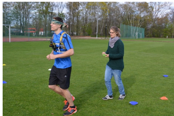
Figure 7: Wizard of Oz experiment evaluating the vibrotactile feedback with blindfolded subjects
