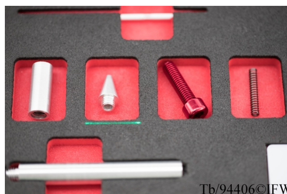
Figure 6: Projection assistance of pick instruction
