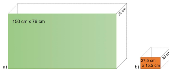
Figure 5: Size of interaction zones. a) Default model. b) Our model for a user with 178 cm body height
