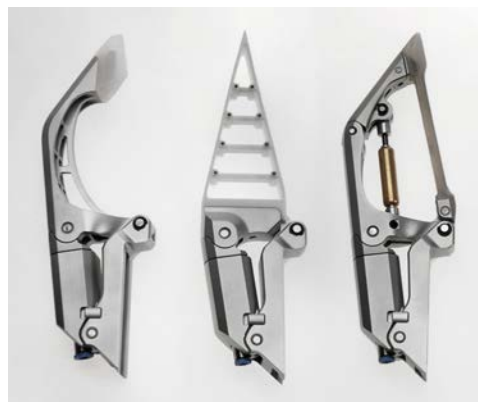
Figure 4: The three jaw modules a) Pincher b) Fish Fin (FFM) and c) Adaptive (AM)
